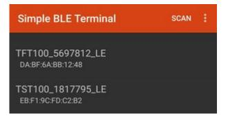
4. After the configuration of device and download of Simple BLE terminal has been completed, open the app and press scan. Select the device with which you are planning to test the functionality from available devices in BLE devices list:
