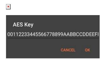
5. Configure the **AES Key** in the **Simple BLE Terminal** by pressing three dots in the top right corner. Use the same **AES Key**, that have been typed in before into **Teltonika Configurator**.
