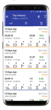
In the history view, you can view all recorded trips. If the trip has was completed with the application still communicating with FMB device – in history it will be marked by the blue line. If the device disconnected during a trip from the FMB for a long period of the timeline will be yellow. Usual cases for trip disconnection could be leaving the vehicle before the trip was completed by FMB configuration. It can be adjusted by Trip parameter Ignition OFF timeout in FMB configuration.
