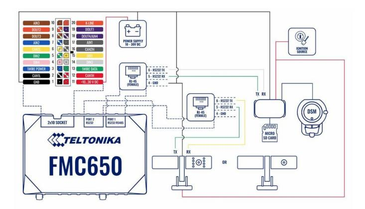
**Two cameras FMC650 Installation with Relay**. If you need to receive additional data from the Two cameras or one of them when the ignition is off, you can also connect the camera to a power source using the relay, to control the power supply by turning on/off the camera. To find information on how to configure DOUT, please visit <u>FMB DOUT</u>.
