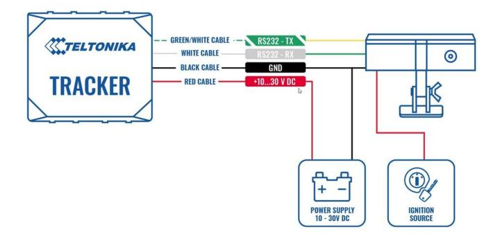
If you need to receive additional data from the DashCam when the ignition is off, you can do it by connecting the camera to a power source using the relay, to control the power supply by turning on/off the camera. To find information on how to configure DOUT, please visit <u>FMB DOUT</u>.
