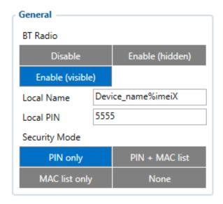
General functionality configures Bluetooth to work in slave mode. This mode allows any external device to connect to FM3001.
