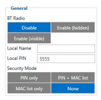
General functionality configures Bluetooth to work in slave mode. This mode allows any external device to connect to FMC150.
