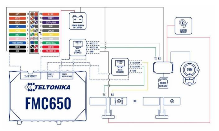
**Two cameras FMC650 Installation with Relay**. If you need to receive additional data from the Two cameras or one of them when the ignition is off, you can also connect the camera to a power source using the relay, to control the power supply by turning on/off the camera. To find information on how to configure DOUT, please visit <u>FMB DOUT</u>.
