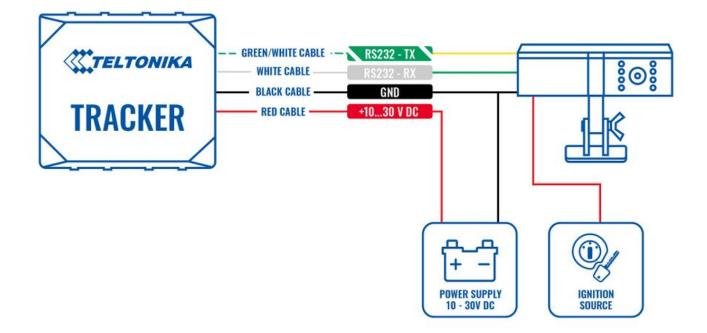
If you need to receive additional data from the DualCam when the ignition is off, you can do it by connecting the camera to a power source using the relay, to control the power supply by turning on/off the camera. To find information on how to configure DOUT, please visit <u>FMB DOUT</u>.
