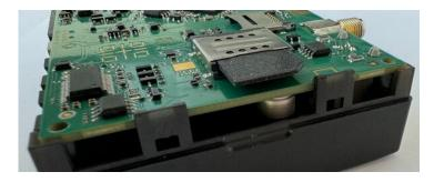
Devices ordered with client SIM cards will have both the 'dummy' SIM card in the top (SIM2) slot and the client SIM card in the
