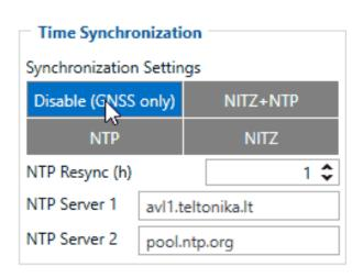
*Synchronization settings* is used for choosing the device's internal time synchronization source.
