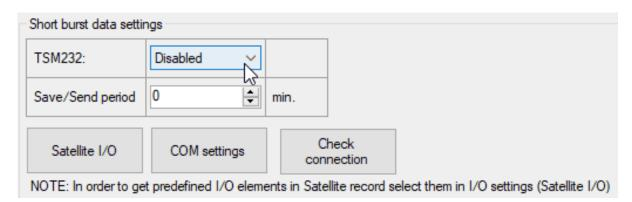
In addition, you can select which IO element can generate Satellite records. In order to do that you need to go to the IO tab select IO record priority Panic and check the checkbox "Satellite I/O" for what you want to get that data through satellites if there is no GSM connection.
