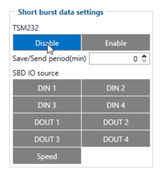
In addition, you can select which IO element can generate Satellite records. In order to do that you need to go to the IO tab select IO record priority Panic what you want to get that data through satellites if there is no GSM connection.
