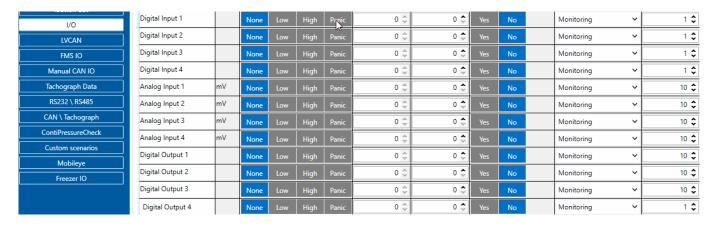
In the scenario shown in the above picture when a panic record is made (generated by Digital Input 1 or Digital Input 2) internal 90 seconds timer will start to tick and if that timeout device will not send a record through the GPRS network it will be sent with Iridium satellites. 9 elements can generate Alarm priority records in the current (00.02.05) firmware version. These elements are:
