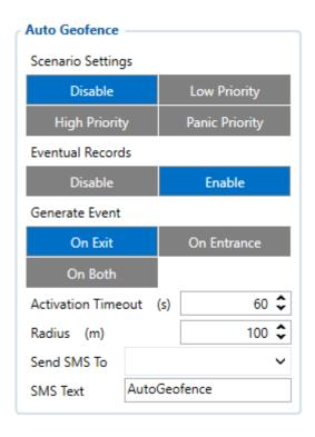
*AutoGeofence* is based on the last known position after the movement has stopped. You can be notified using this function if your device leaves certain area. The shape and size of Geofence zones are set by parameters. It is possible to state whether entering or leaving the geofence triggers an asynchronous message. AutoGeofencing options can be configured by following parameters:
