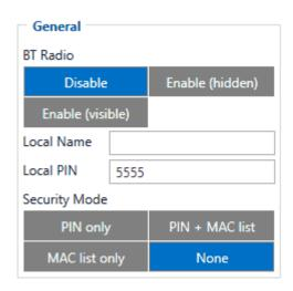
General functionality configures Bluetooth to work in slave mode. This mode allows any external device to connect to FMC1YX.
