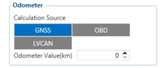
Calculation Source allows to choose Odometer calculation source between GNSS, LVCAN or OBD. Odometer Value sets the starting total odometer value.
