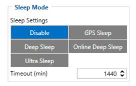
When in GPS sleep mode, FMB640 turns the GPS module off and continues making new periodic records. As a result power usage decreases, in turn saving vehicle battery.
