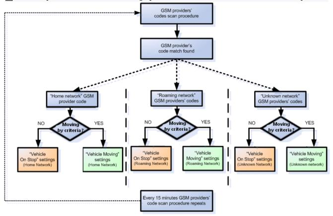
Operator search is performed every 15 minutes. Depending on current GSM operator Home, Roaming or Unknown mode can be changed faster than every 15 minutes. This process is separate from operator search. Movement criteria are checked every second.
