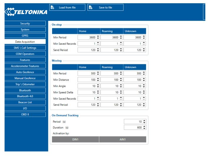
Min Saved Records defines minimum number of coordinates and I/O data that should be transferred within a single connection to the server. If FMB1YX does not have enough coordinates to send to the server, it will check again after a time interval defined in Send Period field.
