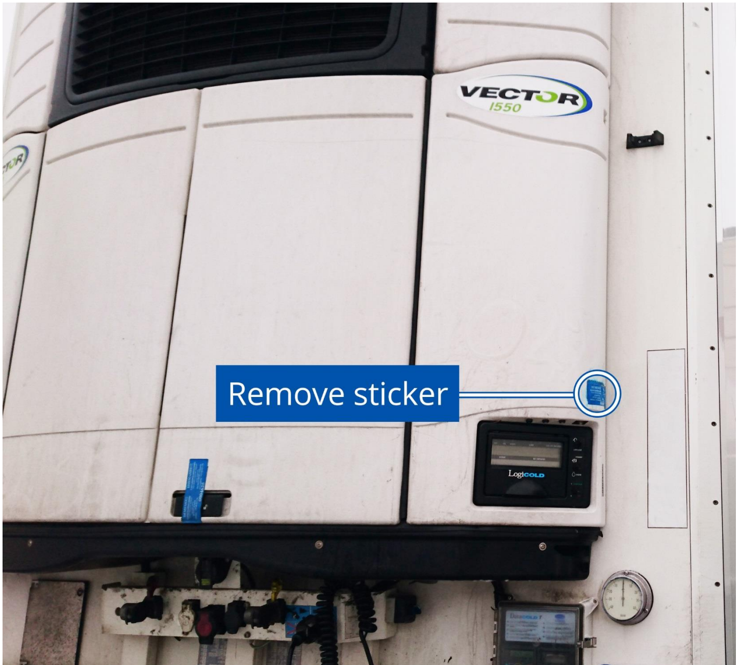
Figure 2 Fuse panel stickers location
