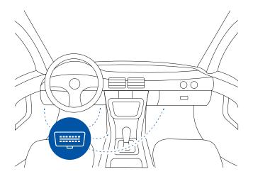
Most common OBDII connector locations.
