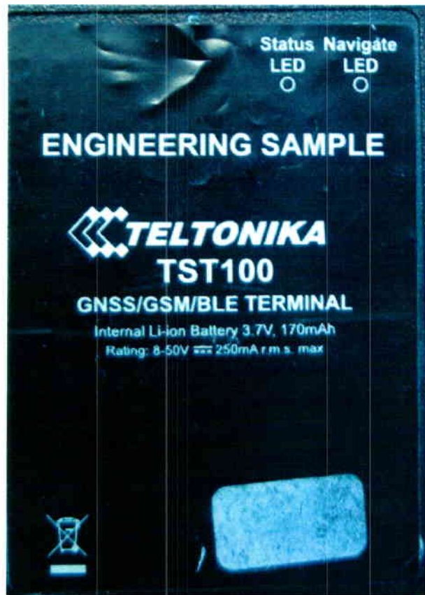
Figure 2. Marking of the scoter tracker housing TST100
