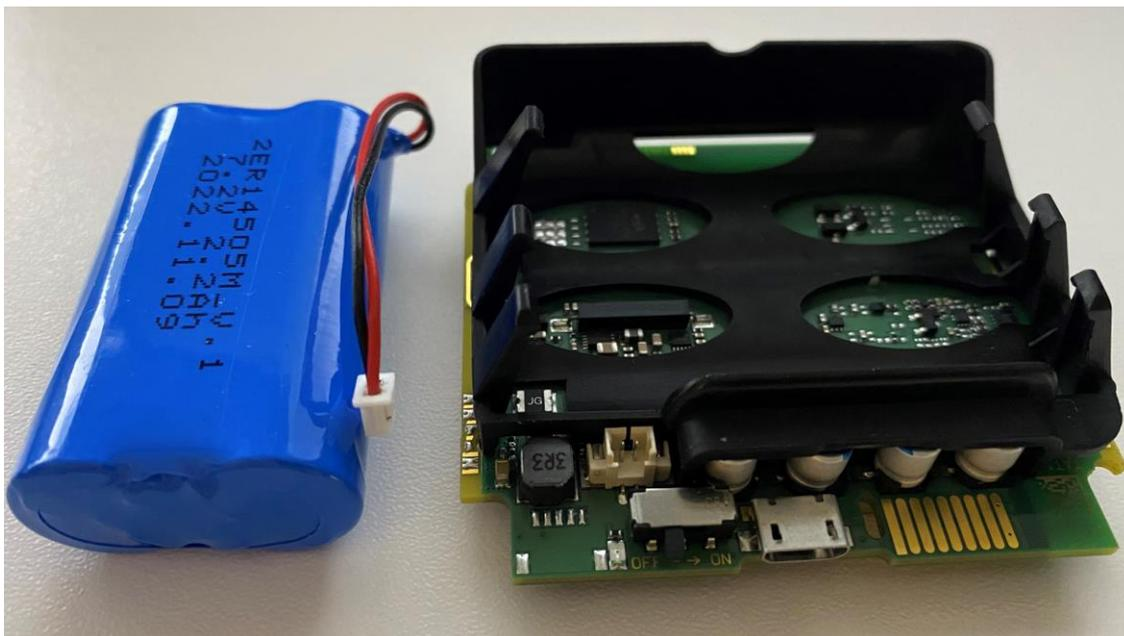
5. Place the new battery with cables facing the same way and connect it
