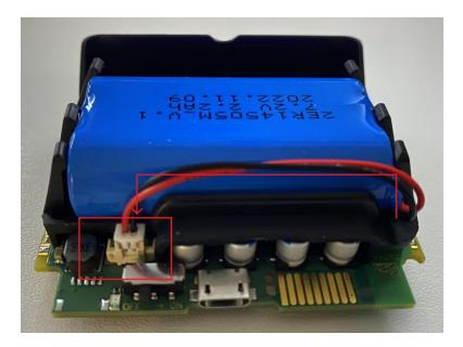
6. Place the PCB back into the housing with GNSS antenna facing the same side as the engraving on the case. Then close the cap.
