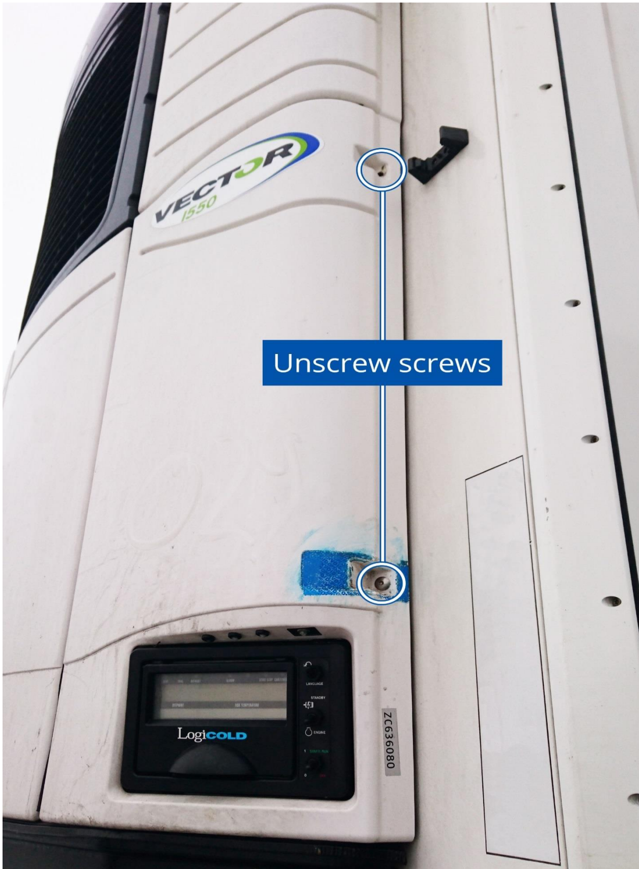
Figure 3 Location of the screws
