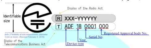
The format of the unique number and CAB ID section differs for radio and terminal equipment.
