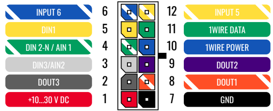
FMM13A 2x6 socket pinout
