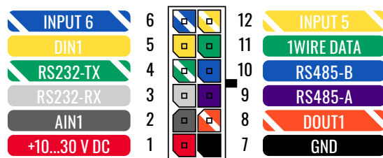
FMM125 2x6 socket pinout
