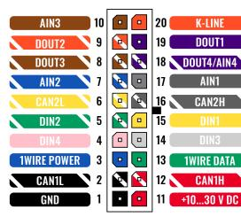
FMC640 2x10 socket pinout
