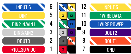
FMC130 2x6 socket pinout
