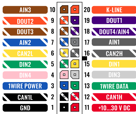
FMC640 2x10 socket pinout
