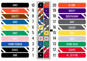
FMC650 2x10 socket pinout
