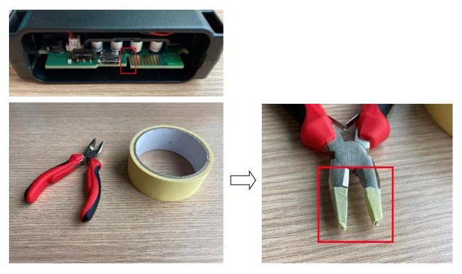
3. Remove the PCB using pliers gripping the shown area, taking care not to damage the contacts
