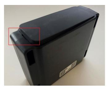
2. Since there is no hole on the PCB we suggest using pliers covered with tape to protect the PCB
