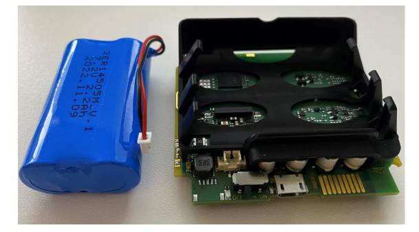
6. Place the new battery with cables facing the same way and connect it
