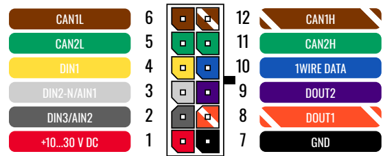
FMM250 2x6 socket pinout
