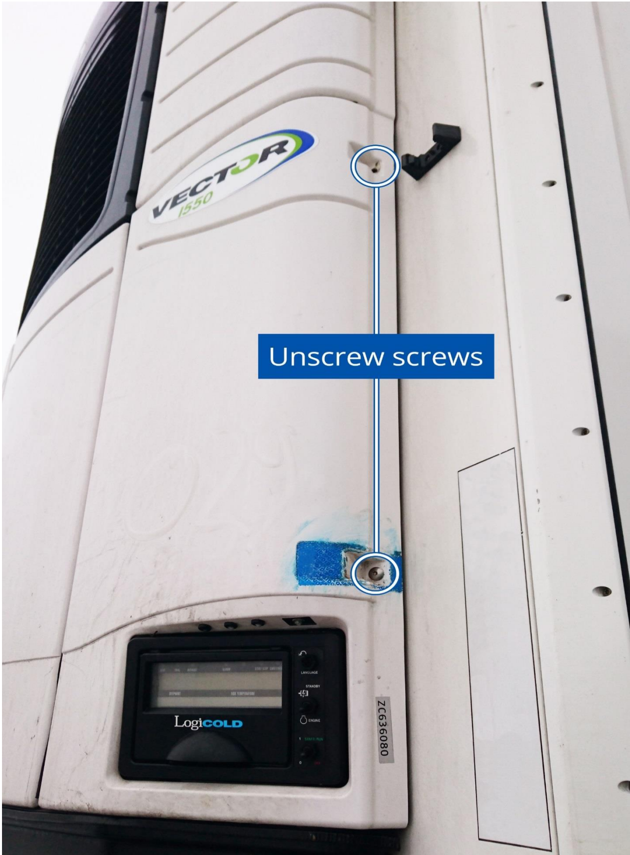
Figure 3 Location of the screws
