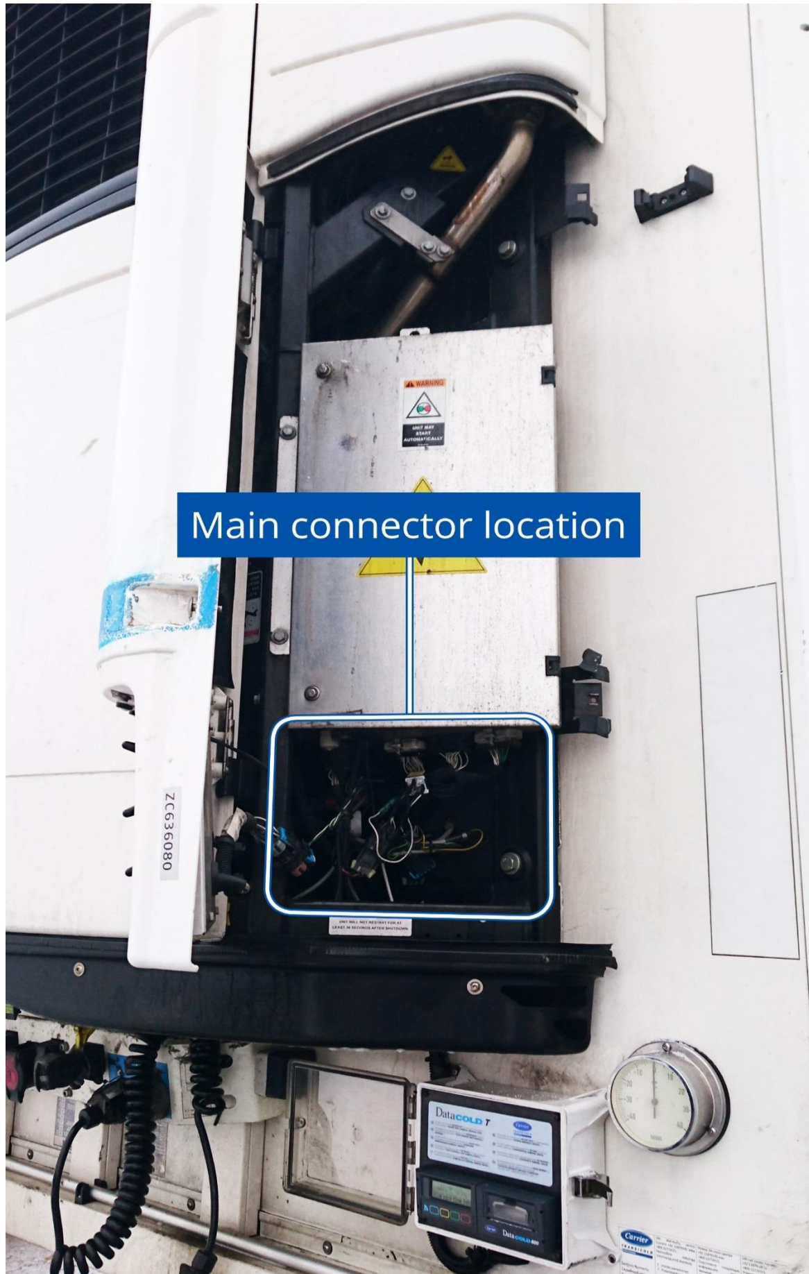
Figure 4 The main connector location
