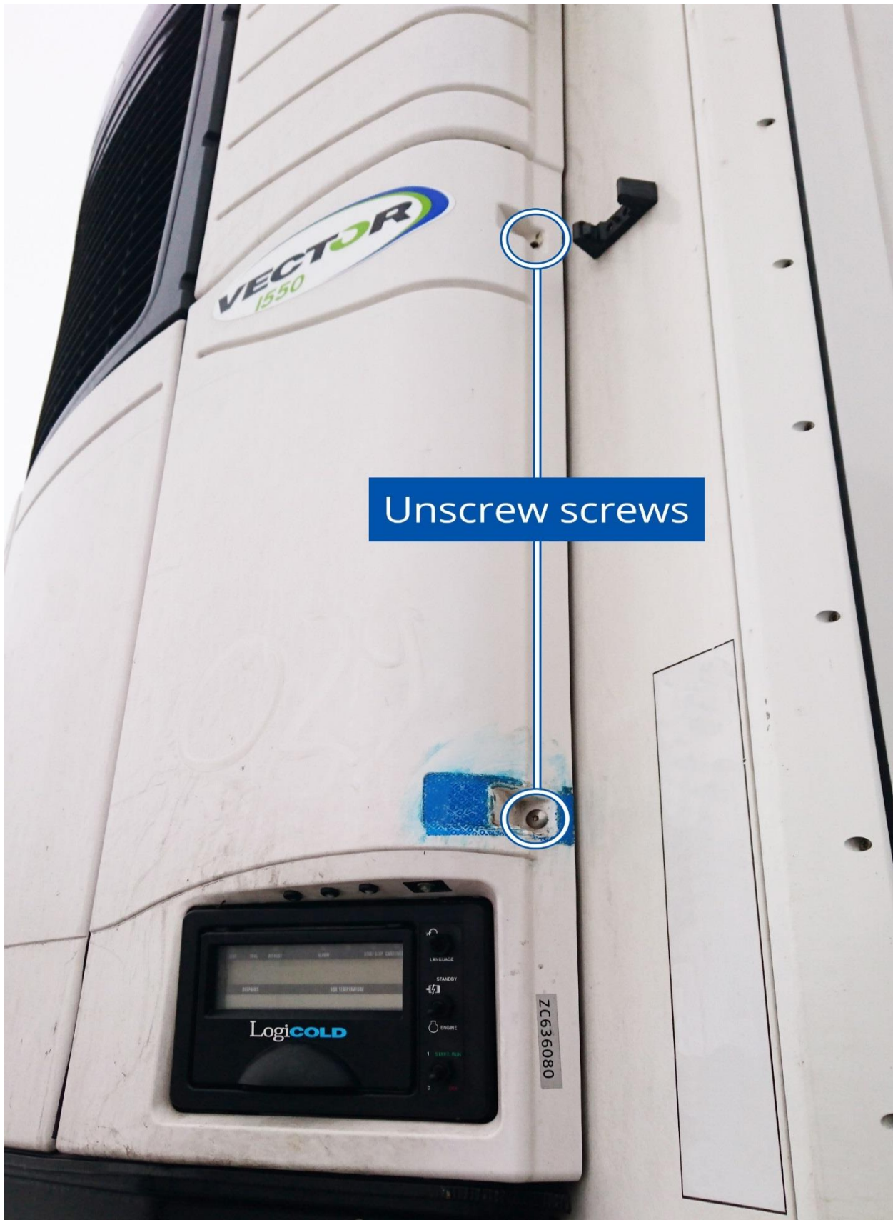
Figure 3 Location of the screws
