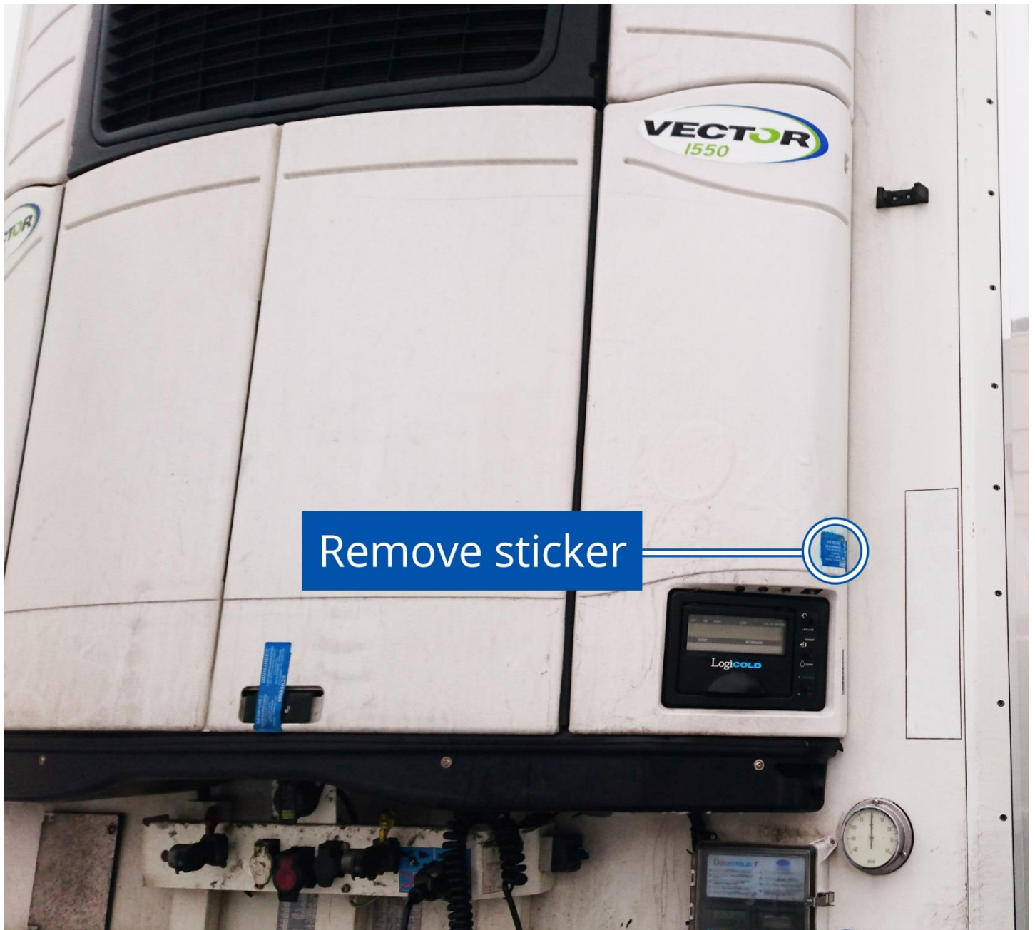
Figure 2 Fuse panel stickers location
