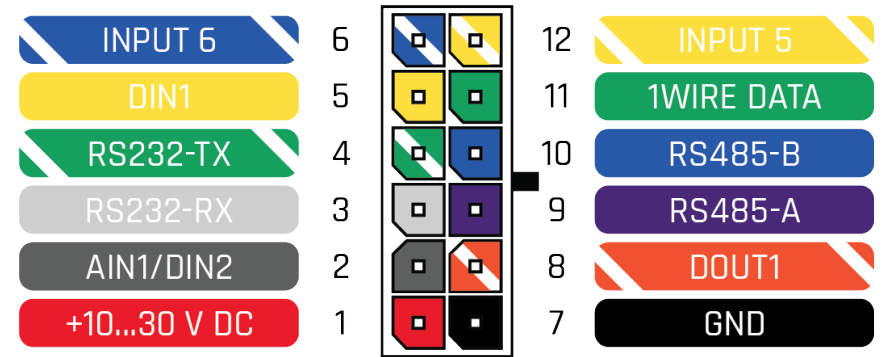
Figure 2 FMC225 2x6 socket pinout
