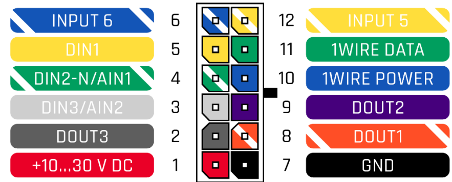
Figure 2 device 2x6 socket pinout
