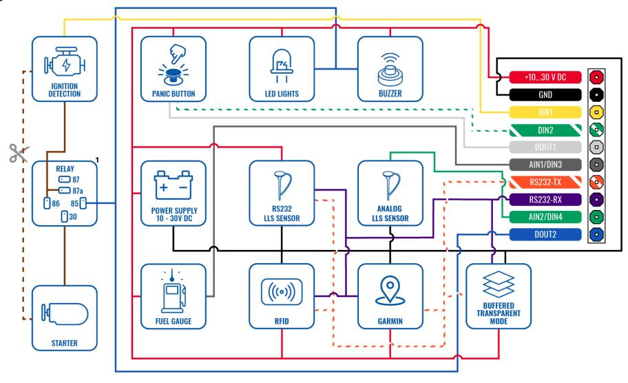
Figure 3 FMB209 Wiring scheme
