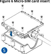
Figure 8 Attaching cover back
