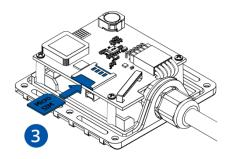
Figure 6 Micro-SIM card insert
