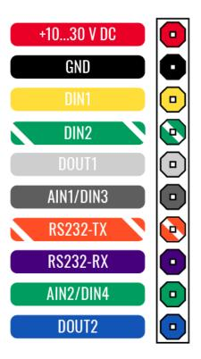
Figure 2 FMB209 Pinout
