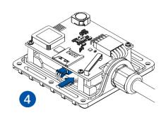
**Figure 7 Battery connection**
