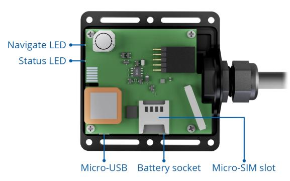
Figure 1 FMB209 device view
