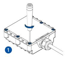
**Figure 4 Unscrew screws**
