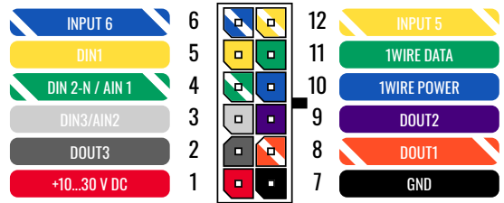
FMC13A 2x6 socket pinout
