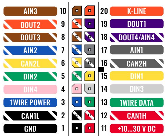
FMC640 2x10 socket pinout
