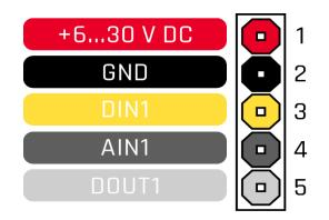
Figure 2 FMB910 pinout
