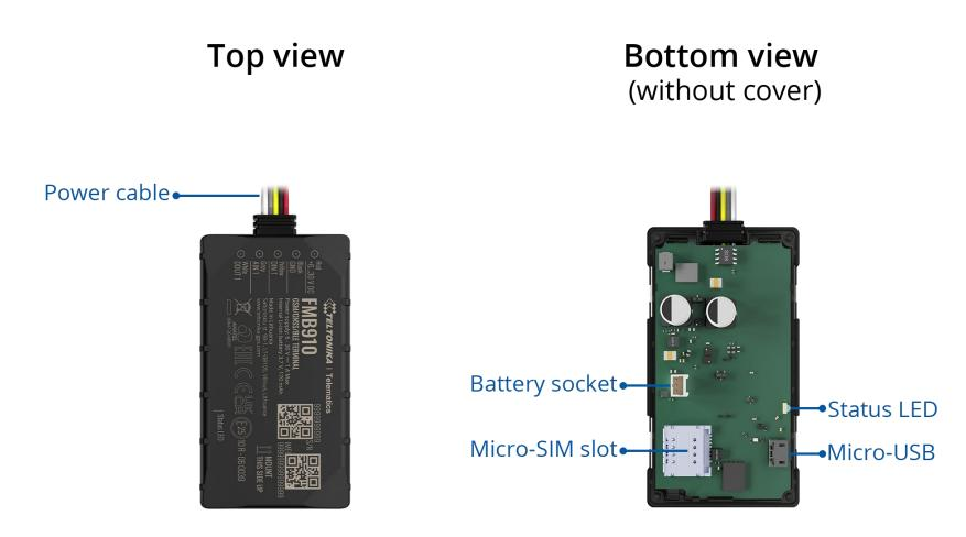
Figure 1 FMB910 device view
