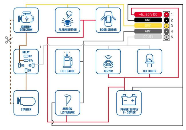
Figure 3 FMB910 Wiring scheme
