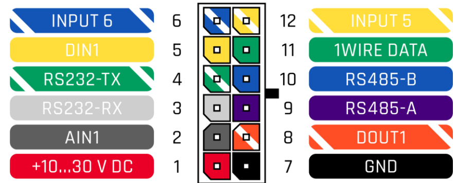
Figure 2 FMB125 2x6 socket pinout
