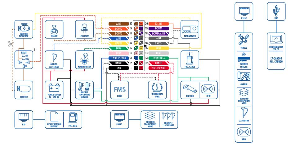
Figure 3 FMB640 Wiring scheme
