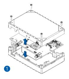
Figure 5 Unscrew screws
