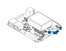
Figure 7 Micro-SIM card insert
