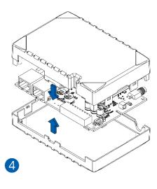
Figure 6 Battery connection
