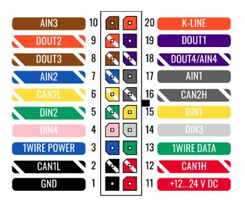
Figure 2 FMB640 Pinout
