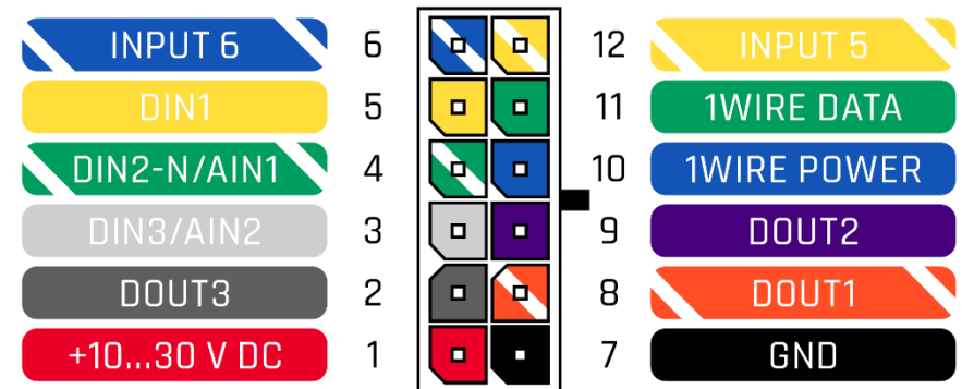
Figure 2 FMM130 2x6 socket pinout
