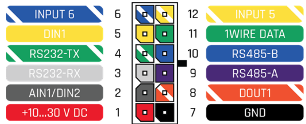
Figure 2 FMM125 2x6 socket pinout
