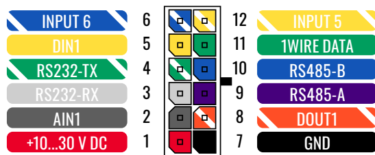
FMB225 2x6 socket pinout
