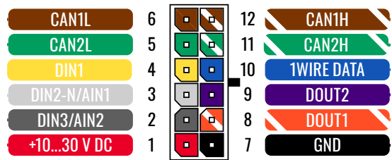
FMB240 2x6 socket pinout
