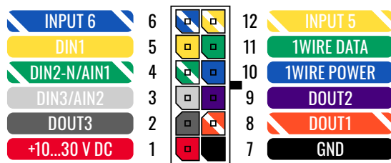
FMM230 2x6 socket pinout
