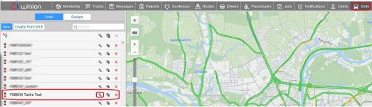
In General tab, press "Configure device for the unit";
