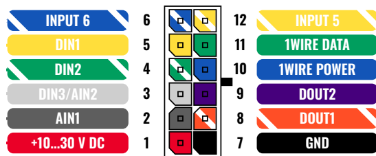
FMB122 2x6 socket pinout
