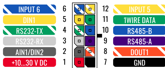
FMC225 2x6 socket pinout
