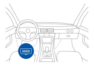
Most common OBDII connector locations.
