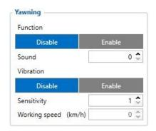
Yawning – this function describes itself, driver yawns, camera event turns on by detecting driver yawning. Function enabling/disabling, sound level, vibration activation, function sensitivity and working speed is configured in the same principle as the functions described previously. Please note, this function does not have automatic transmit function and does not support image and audio sending to server upon activation.
