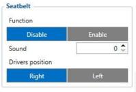
**Seatbelt** – has the function enabling and disabling parameters, adjustable sound level and a selectable driver position which is a useful feature for drivers in countries where they drive on the right side.
