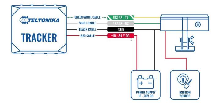
If you need to receive additional data from the DashCam when the ignition is off, you can do it by connecting the camera to a power source using the relay, to control the power supply by turning on/off the camera. To find information on how to configure DOUT, please visit <a href="FMB DOUT">FMB DOUT</a>.
